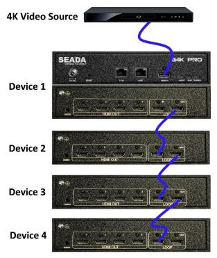
**Note:** the daisy chain HDMI ports only takes the **'processed video source' + 'frame lock'** signals from other G4K Pro. It will not take HDMI video signal from video device directly. Only the main **HDMI IN** port in the front panel is able to take HDMI video signal from video device directly.
